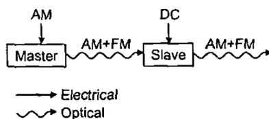
Fig. 1. Schematic of injection-locking with master laser modulation. Master modulation results in slave modulation.
