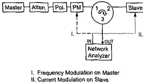
Fig. 2. Schematic of experimental setup for measuring FM-to-AM conversion and direct modulation.
