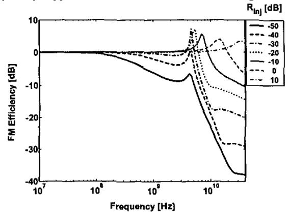
Fig. 9. FM Efficiency for various injection ratios. Driving source: optical FM on master. Measured output: optical FM on slave.
