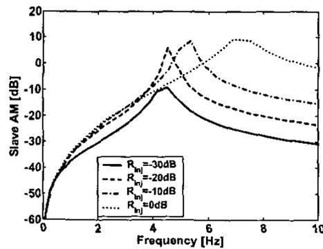
Fig. 5. Theoretical FM-to-AM conversion for various injection ratios
