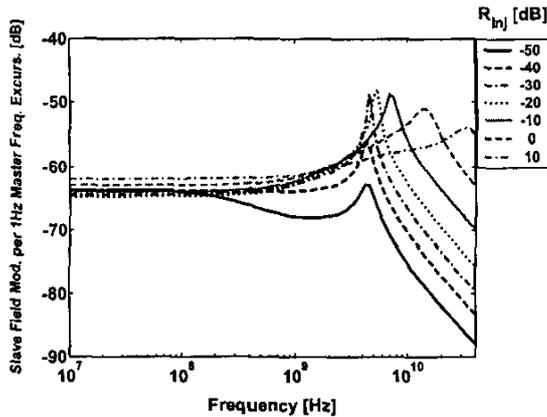
Fig. 8. FM-to-AM conversion for various injection ratios. Driving source: optical FM on master. Measured output: optical AM on slave.
