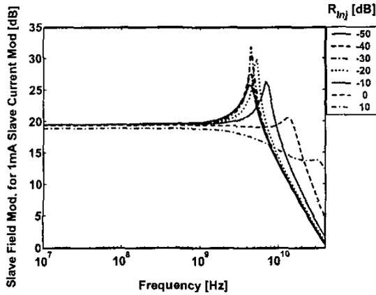
Fig. 6. Direct modulation for various injection ratios. Driving source: Current modulation on slave. Measured output: Optical AM on slave.
