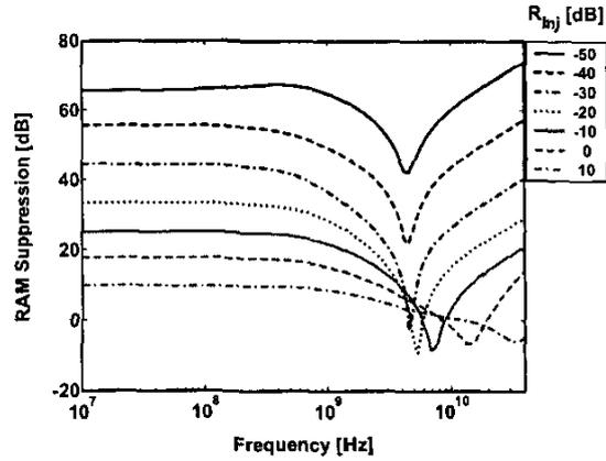
Fig. 7. RAM suppression for various injection ratios. Driving source: Optical AM on master. Measured output: Optical AM on slave.
