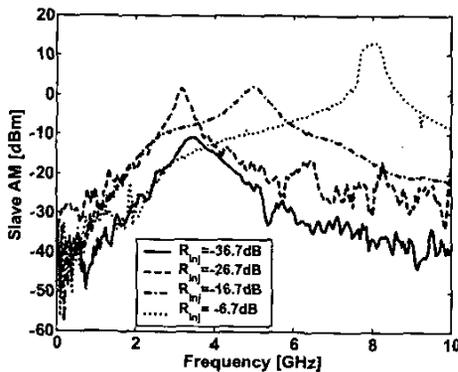
Fig. 4. Experimental FM-to-AM conversion for various injection ratios
