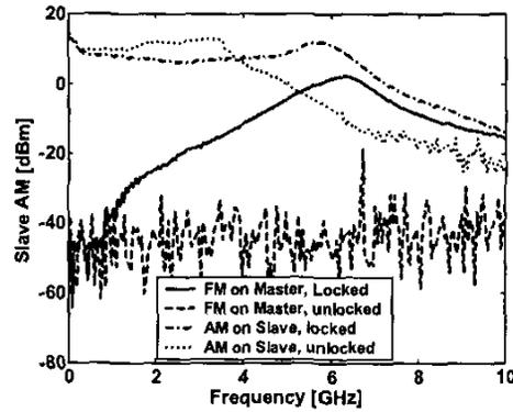
Fig. 3. Slave AM due to different modulation sources. FM-to-AM conversion and direct modulation are shown.
